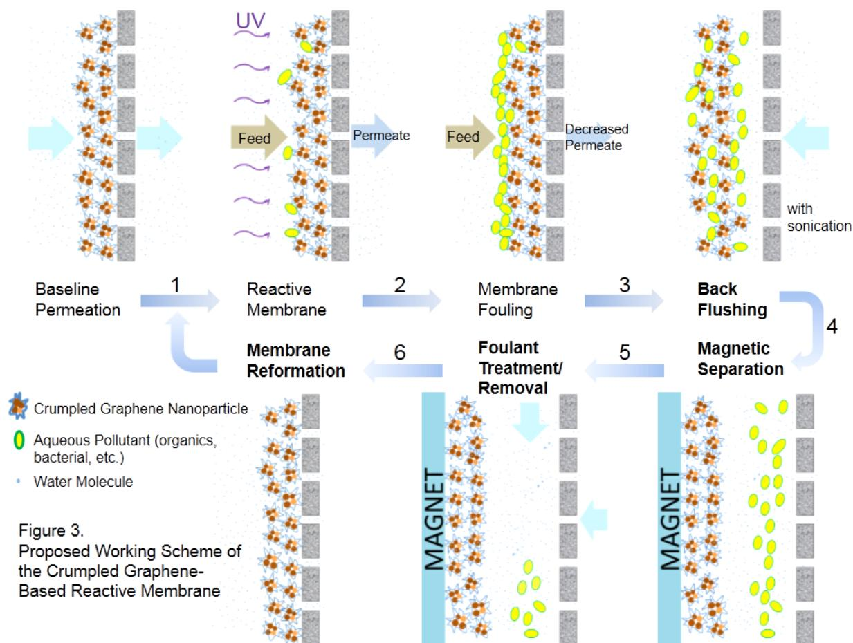
Most water filtration membranes suffer from fouling, or buildup of unwanted material, which necessitates disassembly and cleaning of the membrane. The cleaning process for crumpled graphene oxide nanocomposites would not require full disassembly to remove buildup, and periodic phototreatment regenerates the anti-microbial activity of the Ag
