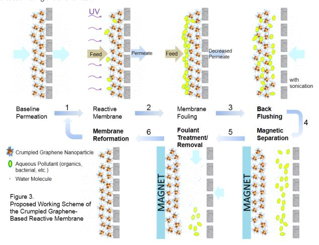
Most water filtration membranes suffer from fouling, or buildup of unwanted material, which necessitates disassembly and cleaning of the membrane. The cleaning process for crumpled graphene oxide nanocomposites would not require full disassembly to remove buildup, and periodic phototreatment regenerates the anti-microbial activity of the Ag
