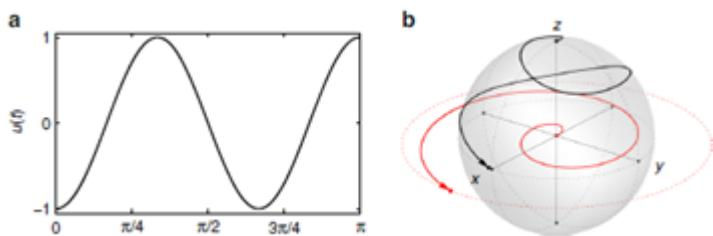
**Exact excitation of single spins.** The minimum-energy control steering the spring (a) with the corresponding trajectories (b) of the spring (red) and spin (black).
