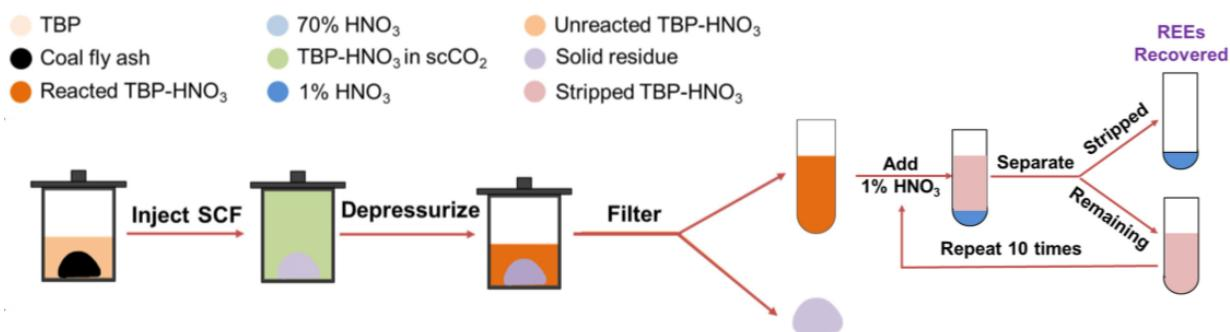
**Overview of the supercritical fluid extraction process from coal fly ash**
