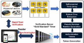
Dynamic hardware-software authentication: combines zeropower timer technology and dynamic authentication software for an enhanced end-to-end security solution.
