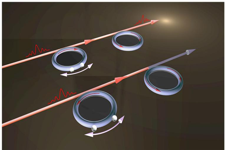
Electromagnetically induced transparency (EIT) is "tuned" by two particles on the optical resonator. The different locations of particles control the propagation of light in either clockwise or counterclockwise directions, which switch on (upper configuration) or off (lower configuration) the interference of light, leading to controllable brightness (EIT) and darkness in the output. Image credit: Yang Lab
