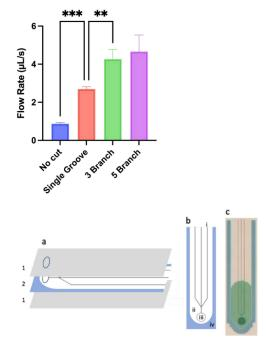
Left: Laser-cut grooves (b, i), branching channels with specialized geometry (b, ii), laser-cut into the filter paper (a, 2), sandwiched between laminate sheets (a, 1) and sealed with wax (b, iv) increases flow rate of  $\mu$ PADs (Right).
