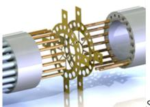
Schematic drawing of bipolar sieve electrode using pins or microwires to interface the contact pads of traditional electrodes fused back-to-back.
