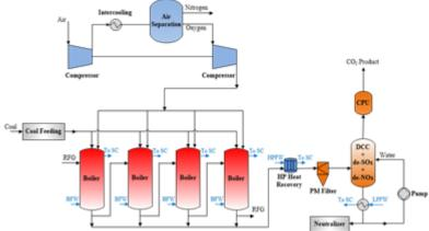
that has been retrofitted with the SPOC process for carbon capture (by adding an air separator unit and other features).
