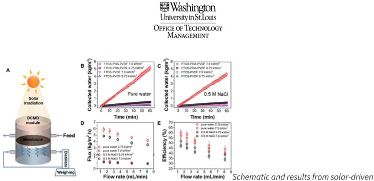
direct-contact membrane distillation (DCMD system) with FTCS-PDA-PVDF membrane
