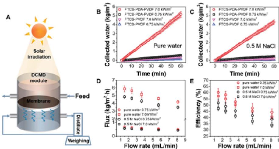
*Schematic and results from solar-driven direct-contact membrane distillation (DCMD system) with FTCS-PDA-PVDF membrane*
