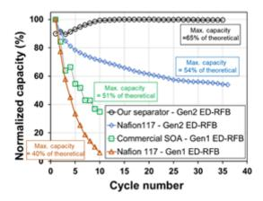
Performance of electrode-decoupled RFB (Gen2) using the AEM separator.
