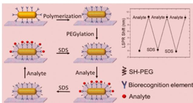
**Schematic of organosilica polymer preservation** – The antibody-covered nanostructure is encapsulated with polymer and then PEGylated. Target analytes bind to the antibodies and are detected through LSPR (localized surface plasmon resonance). An SDS refreshing step releases the target analyte, leaving the antibody available for another capture cycle. The process can be repeated through multiple cycles without compromising sensitivity or specificity.
