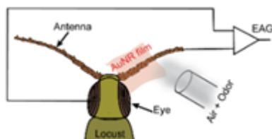
**Schematic of plasmonic nano-tattoo:** The nano-tattoo (AuNR film) is transferred to the insect (shown on the antenna but could also attach to a compound eye or wings), the tattoo can then steer the insect and/or be functionalized to detect specific odors.
