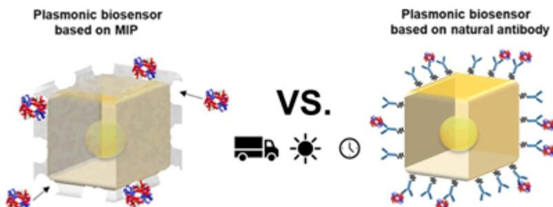
*“MIP” (molecularly imprinted polymer) artificial antibody detection cavities on nanostructured plasmonic biosensors are more stable than natural antibodies after exposure to environmental stressors such as temperature and humidity.*
