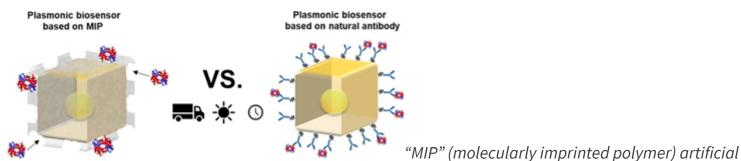
antibody detection cavities on nanostructured plasmonic biosensors are more stable than natural antibodies after exposure to environmental stressors such as temperature and humidity.
